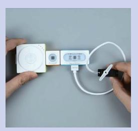
**Offline mode:** Each Neuron module has an independent chip and a unique function. It has some default features via factory settings. Therefore, once user opens the package,the product is readily connected to the module to achieve some simple functions, such as "light sensor + power + display = light value of the current environment"; "gyro + power + LED screen = small ball game, etc.;
